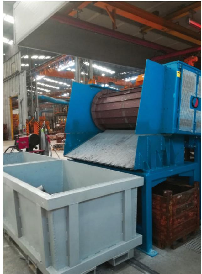
Sprues, runners and gates are, instead, conveyed and discharged into two bins to be then used to feed the furnace.
