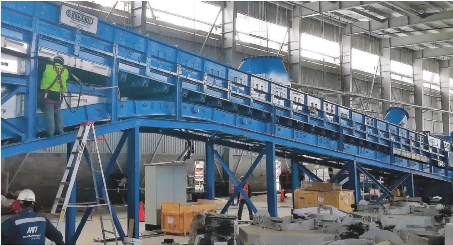
The SuperMCC® has been designed to cool castings down from an inlet temperature of 600 °C to an outlet surface temperature of  $\leq 100$  °C thanks to an optimized cooling process. In fact, equipped with an air forced cooling tunnel held under negative pressure by a venting system, the SuperMCC® guarantees improved performance by means of an additional cooling air flow (cross flow) passing through specifically designed slots on the pans of the conveyor, that increases the cooling rate.
