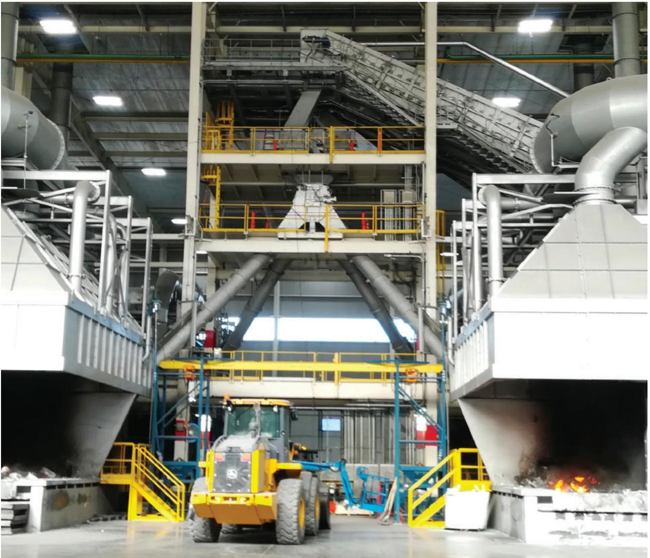
Usually employed to convey hot shreds, conventional apron-based conveyors enclosed in casings are not able to avoid heat dispersion.
