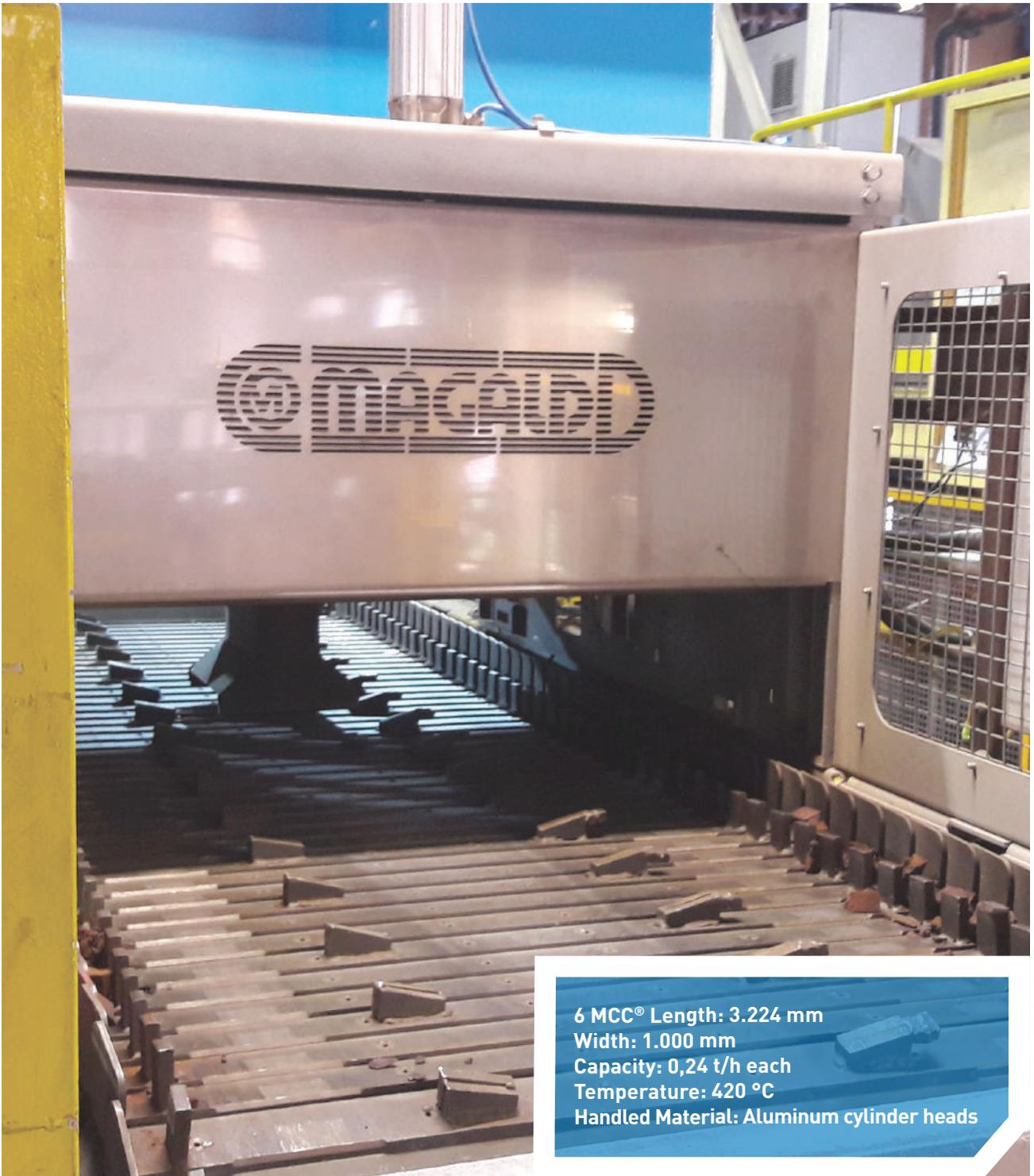
“batch” mode. Loaded by a robot equipped with a gripper, the belt automatically conveys castings inside the cooling tunnel. When they reach a given point inside the tunnel, the belt is stopped again and the pneumatically actuated gates are closed in order to perform the castings cooling.
