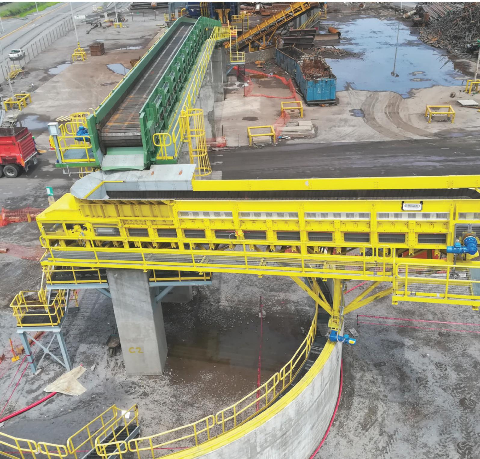
nally, both sides of the conveyor channel are lined with wear resistant plates in order to minimize friction and material jamming.
