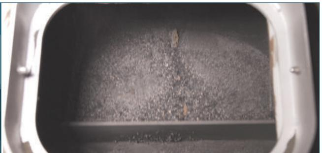
Bottom ash (extinguished and dry) on secondary conveyor Superbelt®
