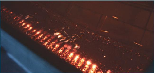
MAP® Post-combustion on the Superbelt® (inclined section)
