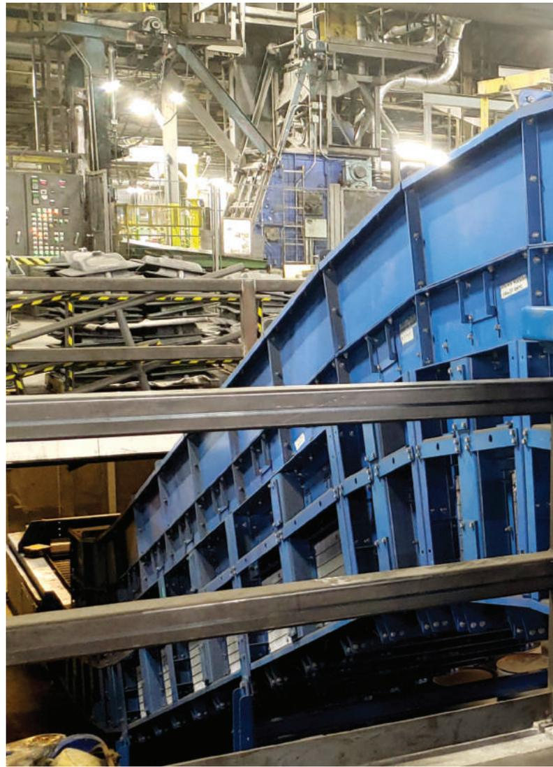
made in manganese steel and designed to have a high impact resistance.
