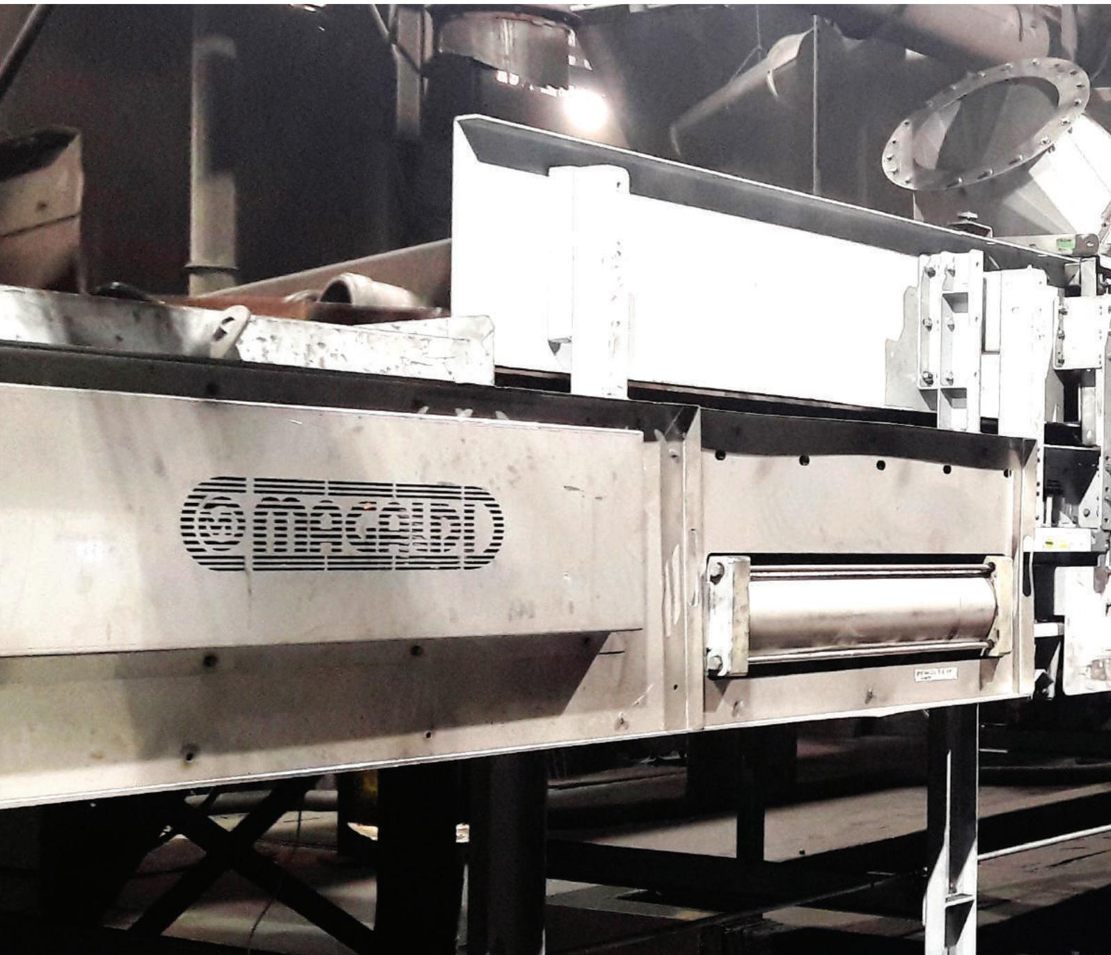
are discharged on the MCC® belt to start the cooling process.
