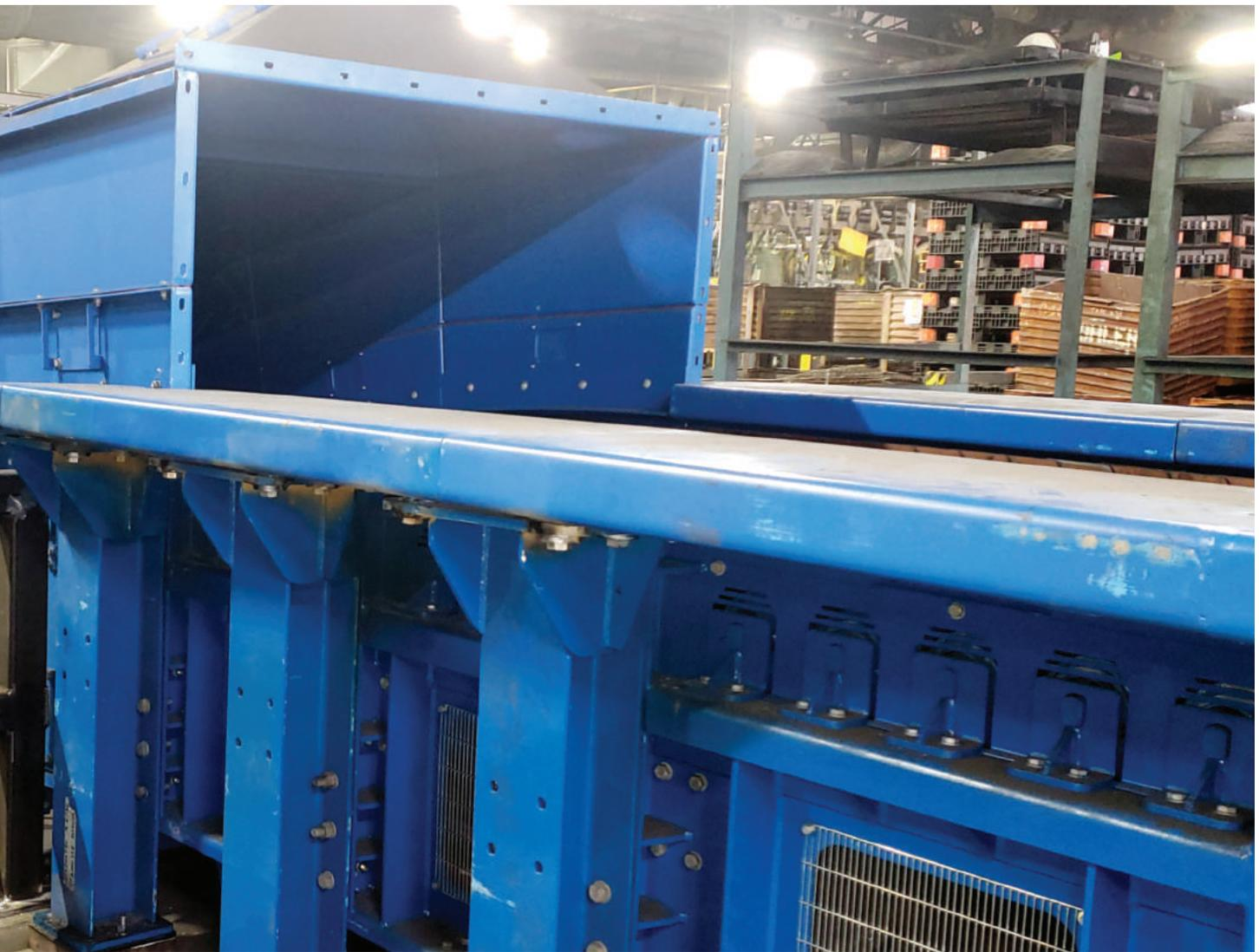
line. To prevent chipping, a special damped chute is installed to absorb the energy generated by the castings impact on it.
