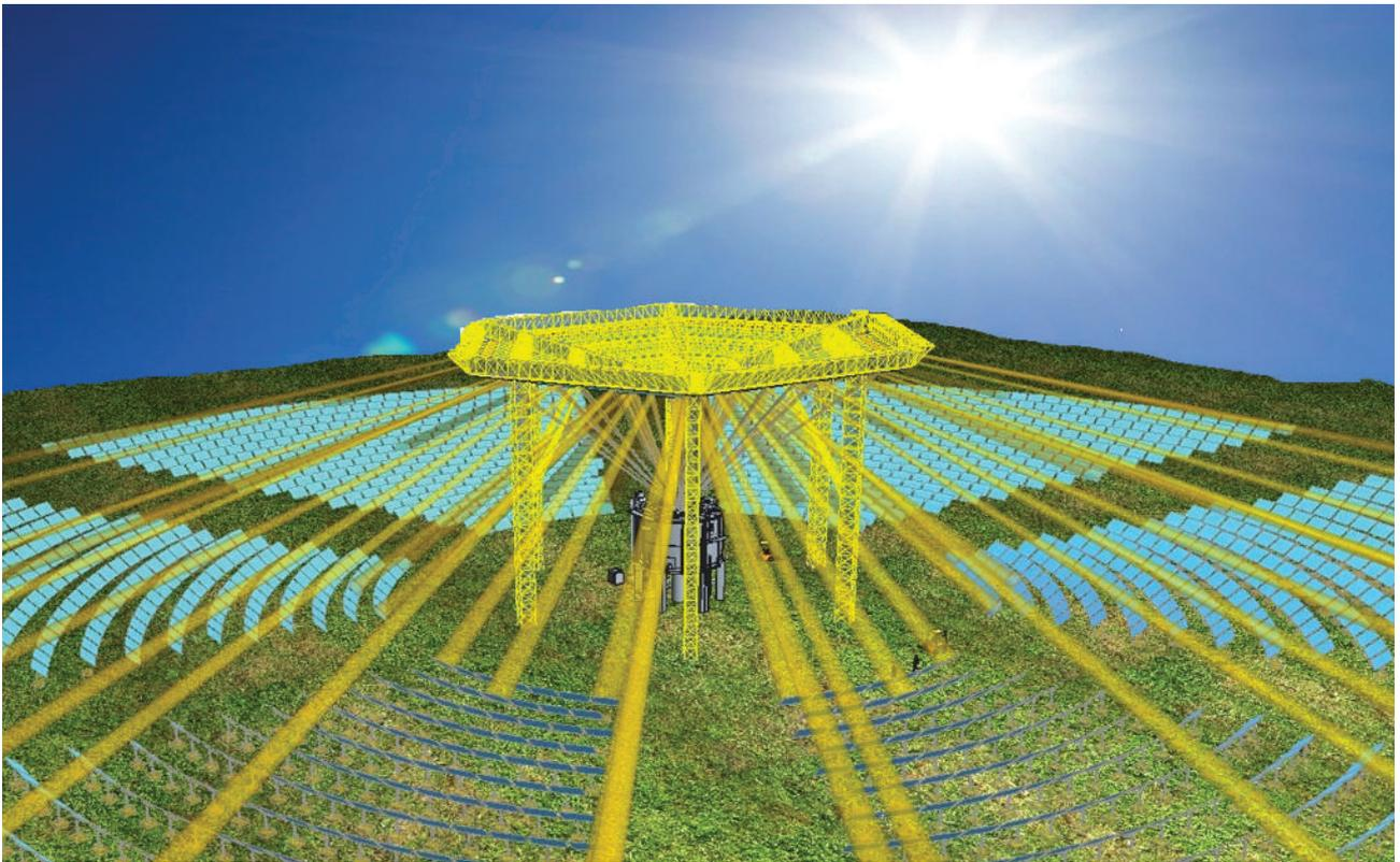
Solar radiation is captured by heliostats and concentrated on a secondary reflector, which directs it into a central solar receiver (MIR) containing a fluidized bed of silica sand. The MIR contains also heat exchangers within the fluidized sand bed for superheated steam generation. The solid particles fluidized bed, directly irradiated
