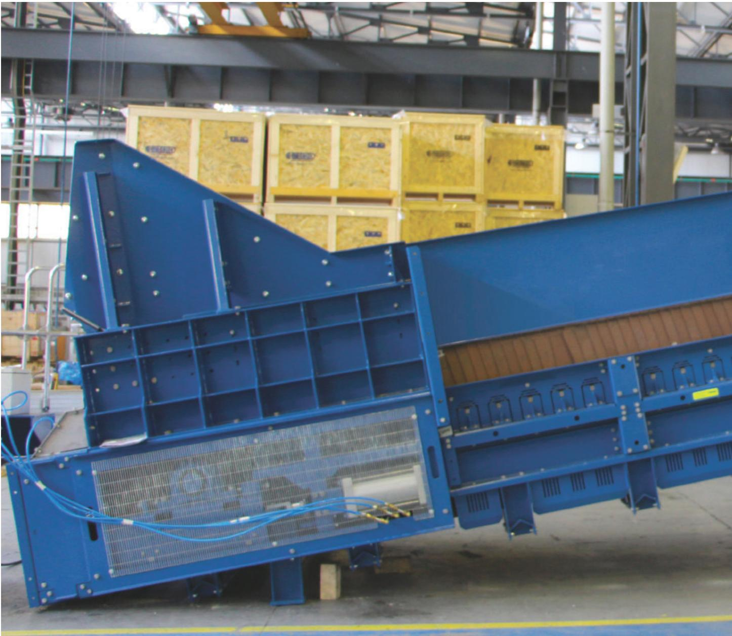
upstream. Proceeding with a belt speed of about 0.05 m/s (to be set by a VFD), the Superbelt® will load the scrap buckets every 60 seconds.
