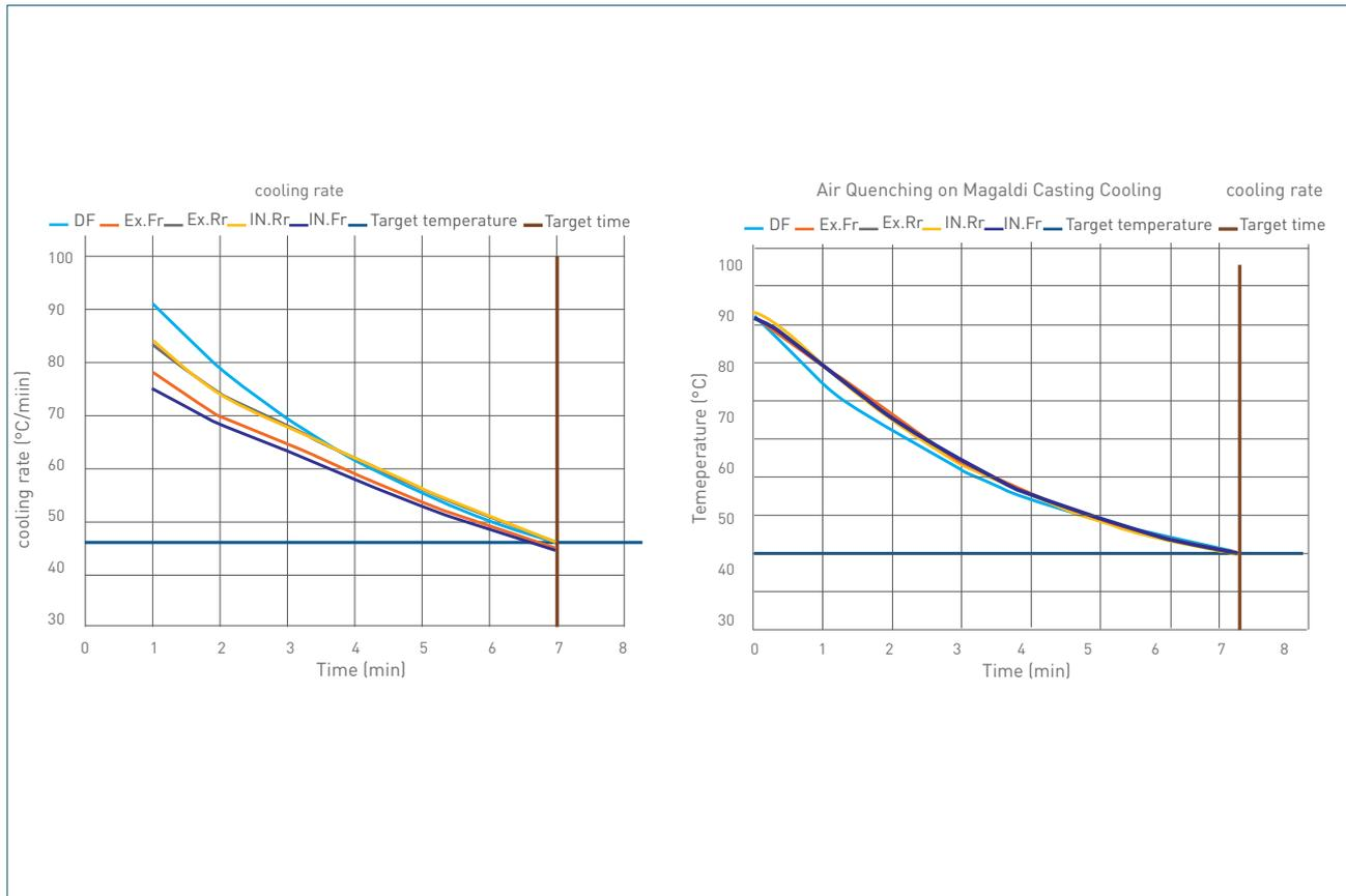
The charts show both the temperature trend and the cooling rate trend over a period of 7 minutes and considering an ambient temperature above 30 °C. Temperature values are measured through 6 thermocouples immersed in the tested casting (used for a destructive test) and recorded by an external data acquisition system.
