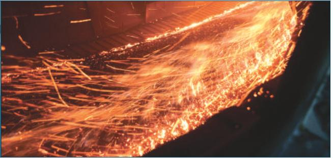
MAP® Post-Combustion on the Superbelt® (after Bottom Ash hopper)
