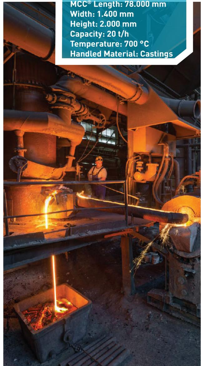
Specifically developed for both a dependable handling/air cooling of castings and the maximum productivity, the MCC® is able to work in the most difficult conditions as high temperatures, heavy loads, abrasive or sharp castings. It can also perform as a valuable workstation for de-gating and sorting operations, avoiding the need for a further conveyor.
