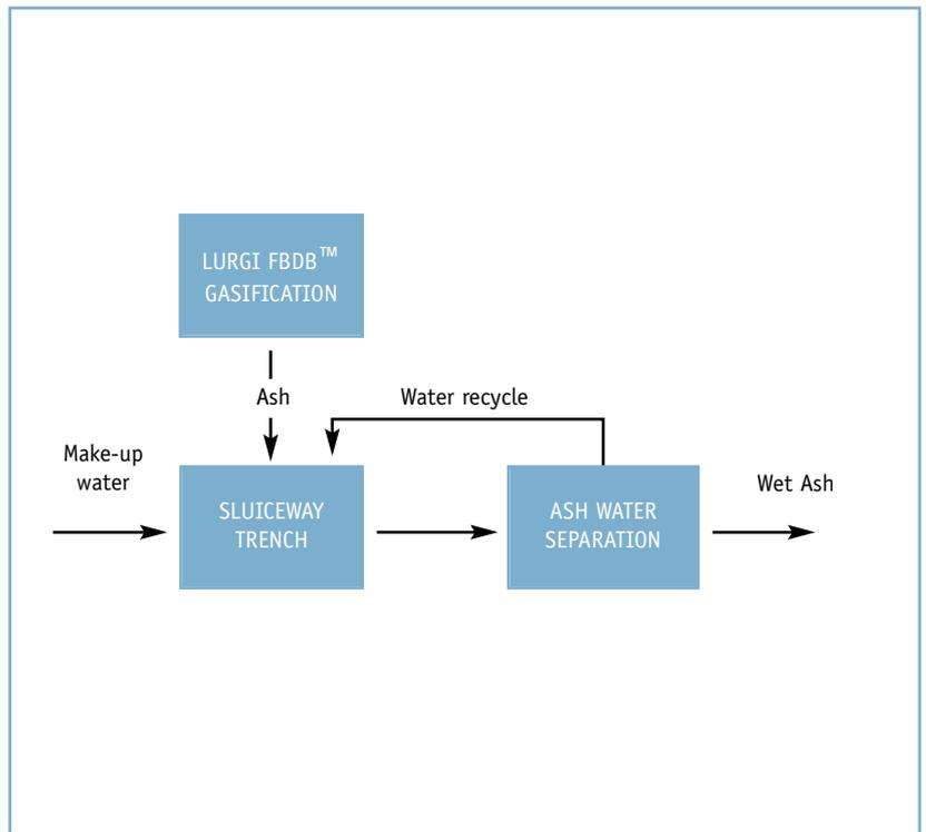
Figure 2: Wet ash sluiceway trench system.
