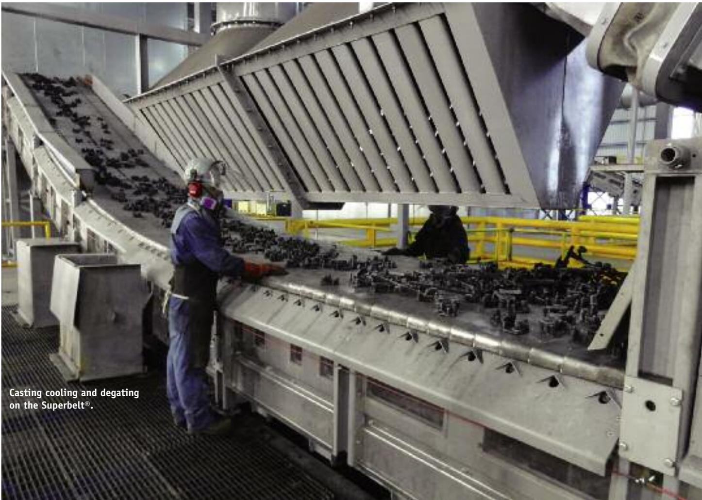
Casting cooling and degating on the Superbelt®.
