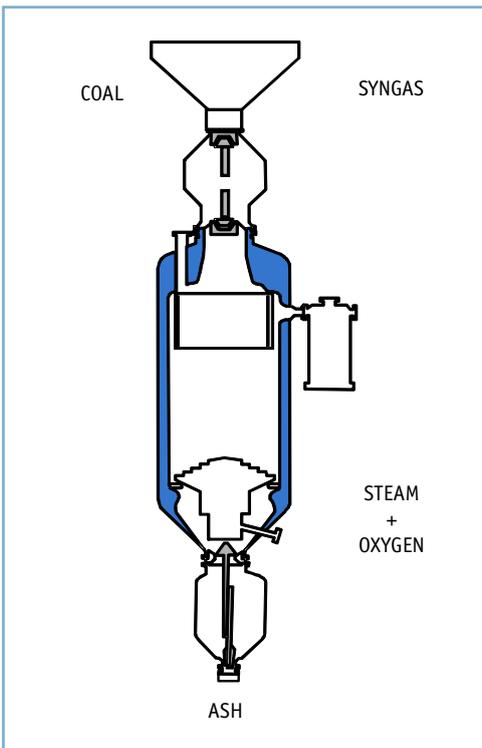
Figure 1: The Lurgi FBDB™ gasification process.
