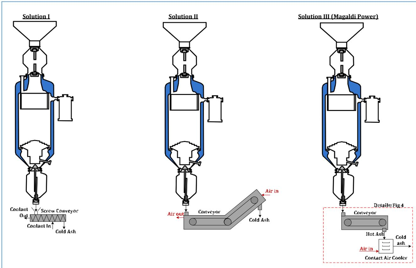
Figure 3: Dry ash handling methods.
