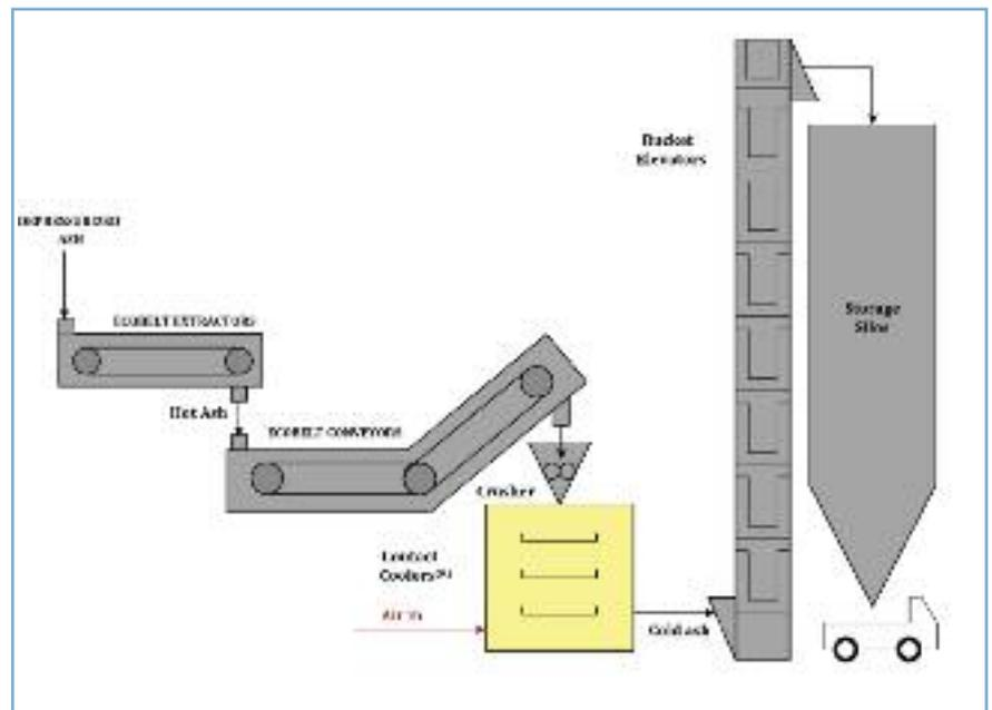
Figure 4: Magaldi Power ash handling process.
