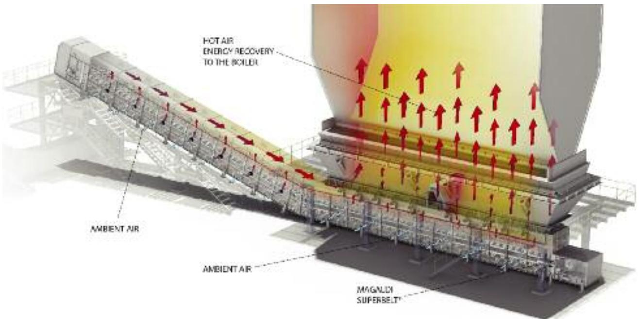
SUPERMAC® system - cross flow cooling.
