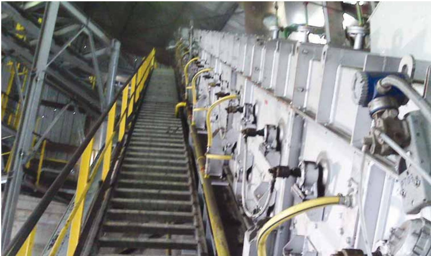
Downstream of the direct reduction process, a further stage may consist of briquetting or smelting hot DRI pellets. In the former case the Magaldi Ecobelt® DRI has the function to cool down the DRI pellets, since the working temperature of the briquetting machine is generally in the range 500÷700 °C. In the latter case the higher the DRI pellet temperature, the higher the energy saving from Electric Arc Furnaces (EAF) to smelt the pellets.
