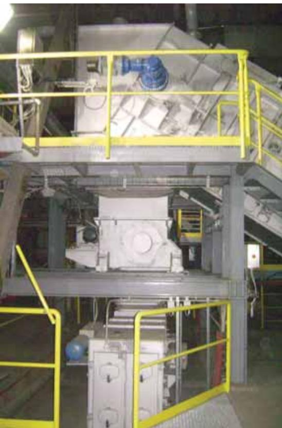
in turn implies a careful selection of the co-fuel preparation system, particularly of its milling stage. High power mills are normally necessary to obtain the suitable small particle size (1-2 mm) required by the combustion process. Due to the physical properties of the biomass, those mills are subject to significant wear and consequently high O&M costs. For the above reasons the selection of the most appropriate bottom ash handling system can be beneficial.
