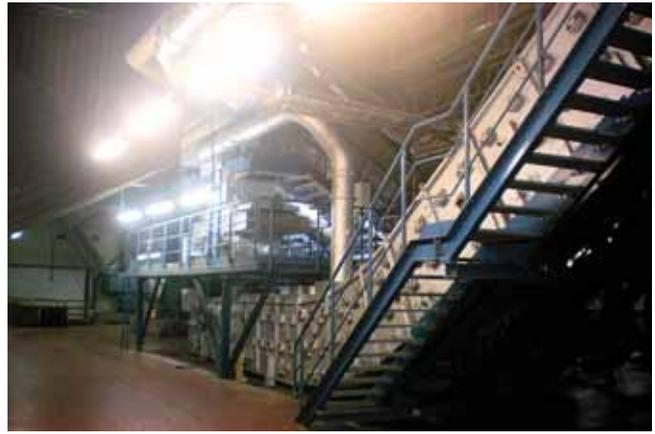
Fig. 4 Postcooler conveyor with crusher station
