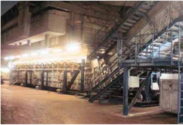
Fig. 3 MAP® - Post-combustor on rails
