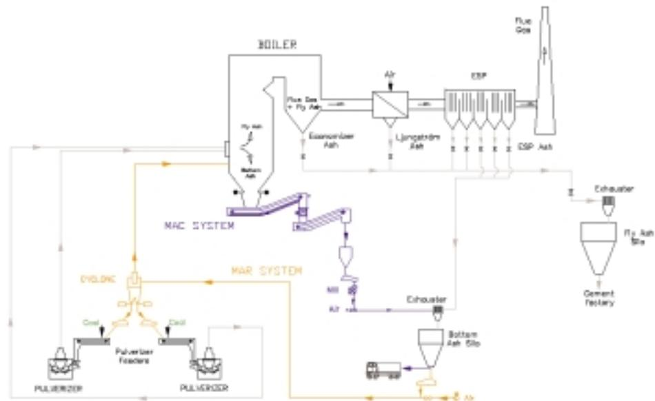
pneumatically conveyed to a cyclone. In the cyclone the finest ash fraction is directly drafted into the combustion chamber due to its negative pressure, while the coarse ash fraction is dosed to the coal feeders and then it passes through the coal pulverizers before being injected into the boiler by the coal burners.
